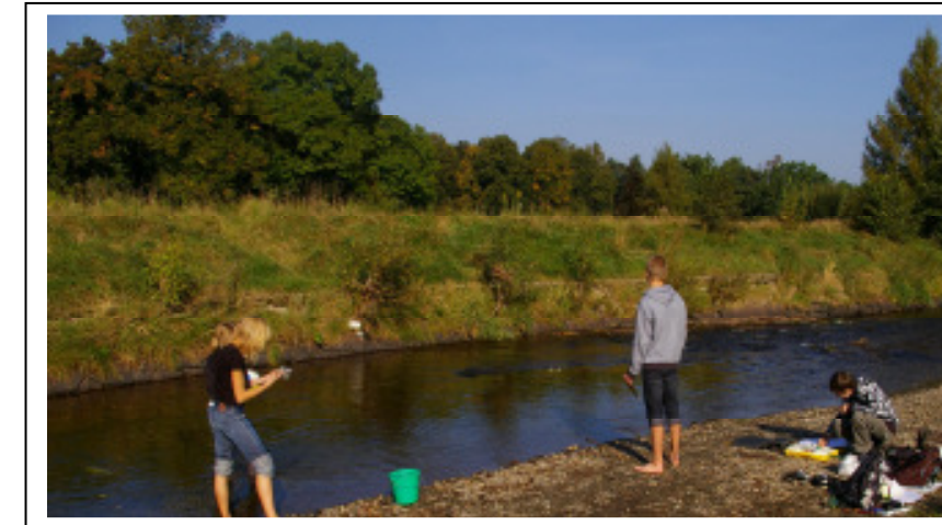
Picture XIX: Measuring the flow capacity by a swimming volleyball
